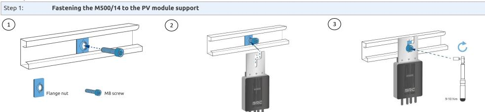
Position the flange nut with an M8 screw into the mounting frame.
