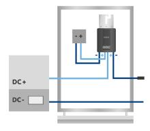
If the module is already connected on the string side, disconnect the connections from the neighboring modules.
