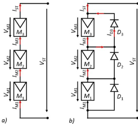
Figure 2: a) Three PV-modules  $M_X$  ( $X = 1..3$ ) connected in series forming a string with voltage  $V_{ST} = V_{M1} + V_{M2} + V_{M3}$ . Currents  $I_{MX} = I_{ST}$  match string current  $I_{ST}$  b) Three PV-modules with antiparallel bypass diodes  $D_X$  in series connection. Bypass diodes  $D_X$  prevent limit of string current  $I_{ST} = I_{M3} + I_{D3}$  in case  $M_3$  becomes partly shaded.
