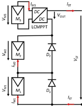
Figure 7: Module  $M_3$  equipped with LCMPPPT connected in series to  $M_1$  and  $M_2$  with bypass diodes  $D_1$  and  $D_2$  result in String voltage  $V_{ST}$ . In case of shade LCMPPPT bucks  $V_{M3}$  to  $V_{OUT}$  and boosts  $I_{M3}$  to match  $I_{M1} = I_{M2} = I_{ST}$  of modules  $M_1$  and  $M_2$ , protected by diodes  $D_1$  and  $D_2$ .
