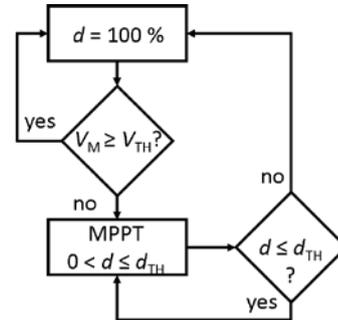
Figure 6: Activation algorithm of MPP tracking. If  $V_{MY} < V_{TH}$ , MPPT activates. When the shade disappears  $d > d_{TH}$  disables the MPPT and  $d = 100\%$  connects  $M_Y$  in series to the modules  $M_Z$ .
