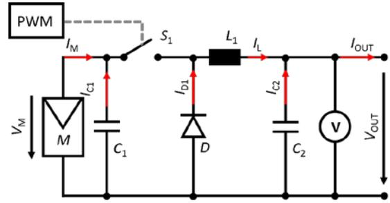
Figure 5: Schematic of LCMPPPT.  $C_1$  and  $C_2$  stabilize  $V_M$  and  $V_{OUT}$ .  $S_1$ ,  $L_1$  and  $D$  forming a buck converter. A PWM signal with duty cycle  $d$  boosts  $I_M$  to  $I_{OUT}$ . Voltage measurement for MPPT
