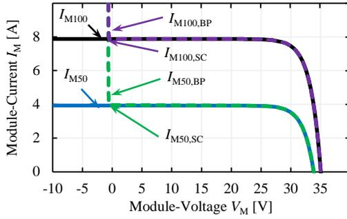
Figure 1: Module current  $I_{M50}$  of 50 % illuminated module without and  $I_{M50}$  with bypass diode.  $I_{M100}$  100 % illuminated module without and  $I_{M100BP}$  with bypass diode. Without bypass diode short circuit currents  $I_{SC,50}$  and  $I_{SC,100}$  limit  $I_{M50} \leq I_{SC,50}$  and  $I_{M100} \leq I_{SC,100}$ . With bypass diodes there is no limit.
