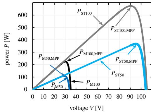
Figure 3: Power  $P_{M100}$ , with maximum  $P_{M100, MPP}$ , of 100 % and  $P_{M50}$ , with maximum  $P_{M50, MPP}$ , 50 % illuminated module. Three modules in series,  $P_{ST100}$ , with maximum  $P_{ST100, MPP}$ , all modules 100 % illuminated and  $P_{ST, 50}$ , with maximum  $P_{ST100, MPP}$  two modules 100 % and one module 50 % illumination.
