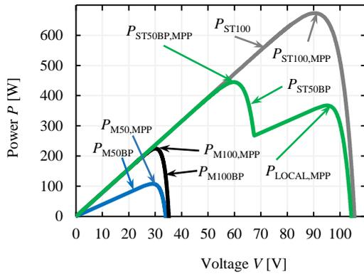
Figure 4: Power  $P_{M100BP}$ , with maximum  $P_{M100BP,MPP}$ , of 100 % illuminated module with bypass diode  $D$ , and  $P_{M50BP}$ , with maximum  $P_{M100,MPP}$ , 50 % illuminated with bypass diode  $D$ . Three modules in series,  $P_{ST100BP}$ , with maximum  $P_{ST100,MPP}$ , all modules 100 % illuminated and  $P_{LOCAL,MPP}$  local maximum  $P_{ST,MPP50}$  and global maximum  $P_{ST50BP,MPP}$  with bypass diode active for two modules 100 % and one module 50 % illumination.
